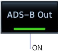
Tapping **ADS-B Out** allows the transmission of ADS-B Out messages and position information.
