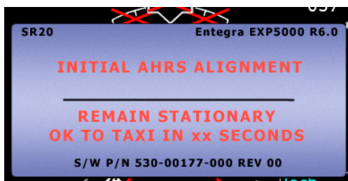
Figure 7. Entegra EXP5000 AHRS Alignment Message
