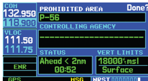
Figure 8-39 Airspace Page for Prohibited Area
