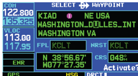
Figure 4-5 Facility Name Selected
